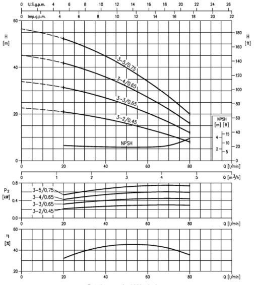
Rotation speed ≈ 2850 min-1 Test standard: |SO 9906:2012 - Grade 3B
